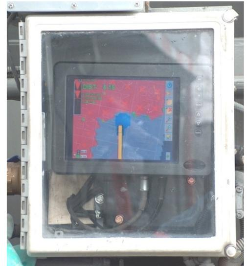
The operator sees the rate of delivery and the progress toward the entered quantity. The plant operator can adjust the rate of delivery to match the rate of mixing progress shown on the screen. When the entered quantity of reagent is reached the system shuts off.
