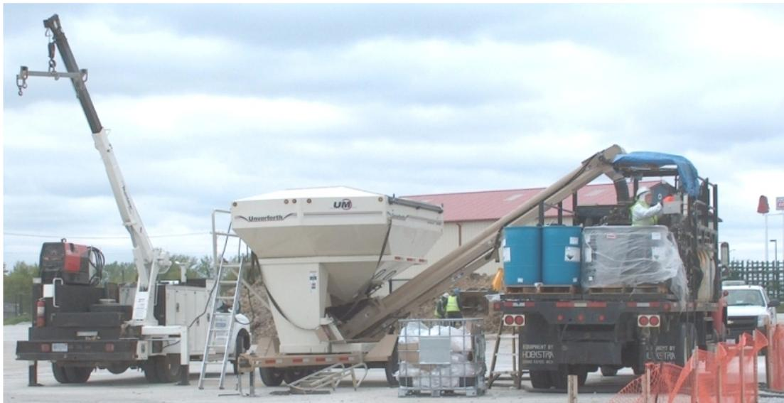
The outgoing quantity of reagent solution is entered. The system will shut the delivery off when the entered quantity is reached. The LTC ISCO reagent delivery plant has been used for persulfate, permanganate, Regenox, Modified Fentons Reagent, Daramend, ZVI & biological reagents.
